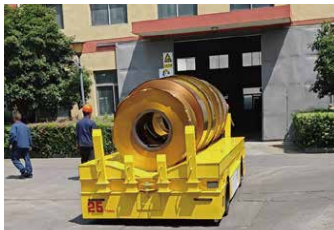
25 tons Trackless flat car+ manual remote control for copper roll.
