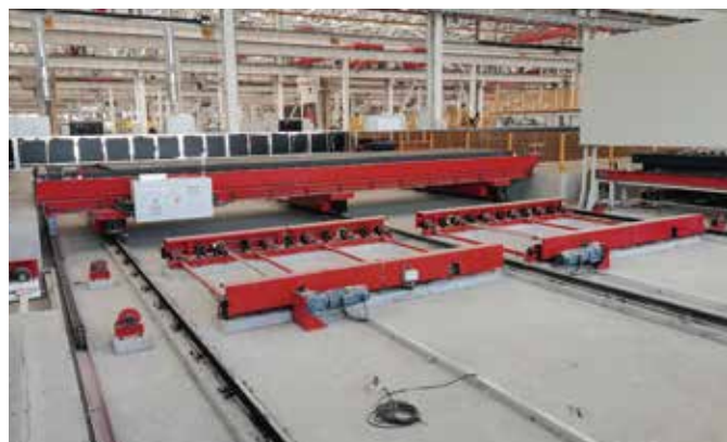
20 tons RGV + Automatic rail replacement for Laser cutting machine blanking.
