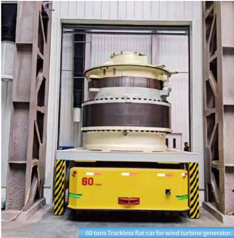
50 tons Trackless flat car for wind generator component.
