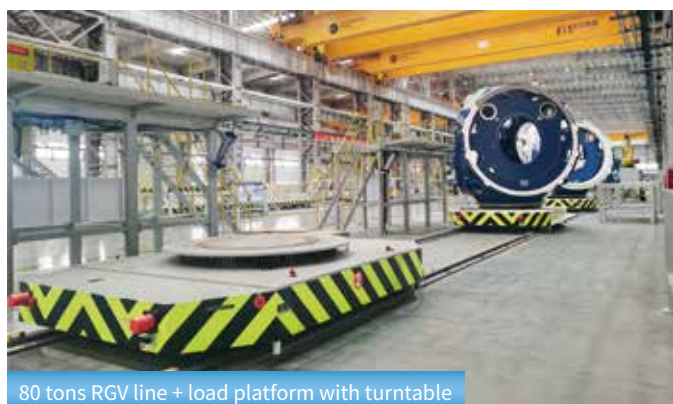
80 tons RGV line + load platform with turntable
