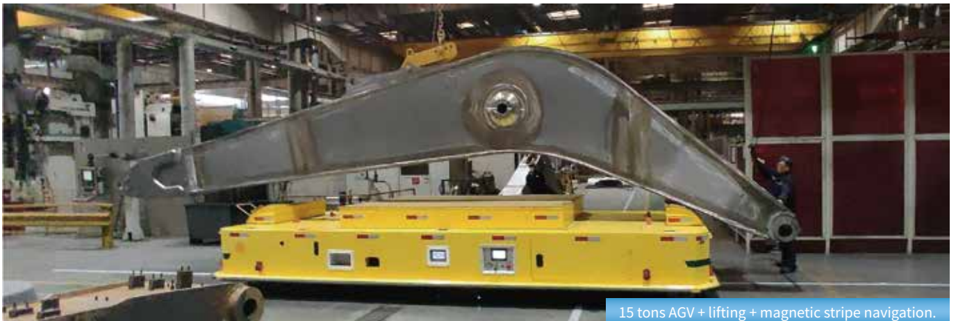
15 tons AGV + Laser & RTK navigation for copper smelting industry.
