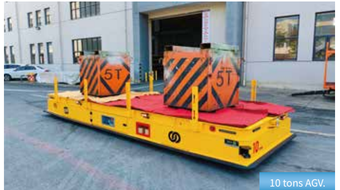
5 tons AGV for production line applications in the automotive industry.
