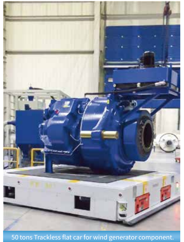
60 tons Trackless flat car for wind turbine generator.
