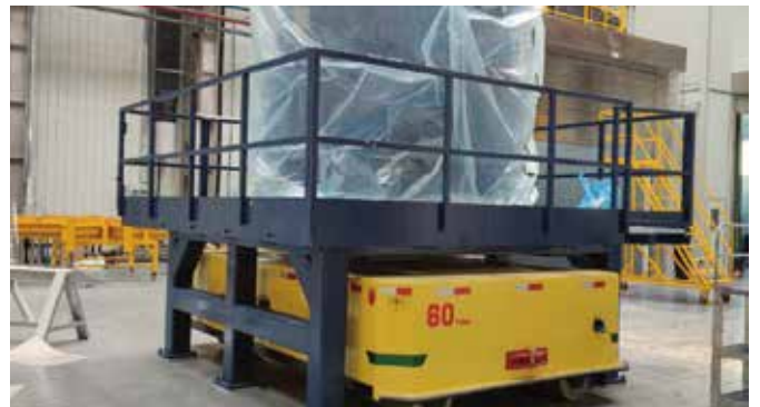
60 tons AGV + latent and lifting back-carried+ magnetic stripe navigation.
