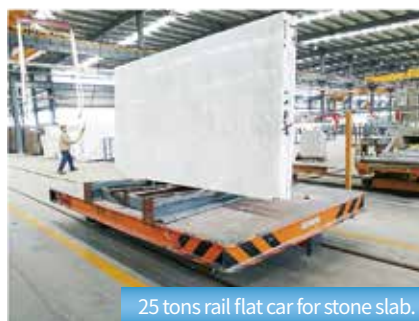
25 tons rail flat car + U type platform.
