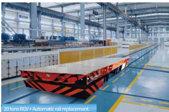
20 tons RGV + Automatic rail replacement for Laser cutting machine blanking.
